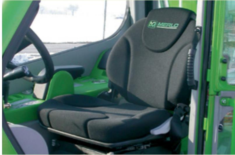
Newly contoured and strengthened, the TURBOFARMER seat is easily identified by the Merlo logo. Fully adjustable forwards and backwards, it also features seat back and seat angle adjustment to comfortably accommodate any driver. As an option, a weight-adjustable air suspension seat isolates the driver from the majority of external vibrations, ensuring productive and safe working, especially during road travel.
